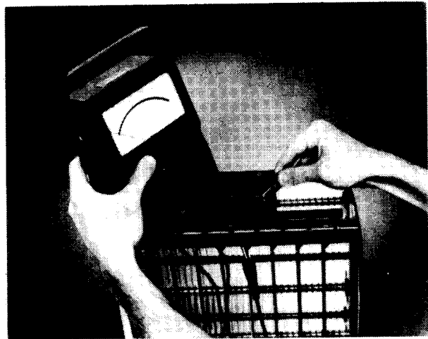
FIG. 11—USE AN OHMMETER TO CHECK THE ELECTRONIC CELLS FOR SHORT CIRCUITS.
